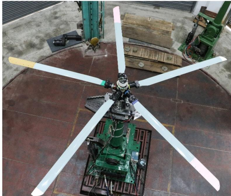
**Figure 1.** Test stand and rotor model.
