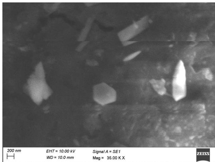
Fig. 4. SEM images of *Tecoma stans* mediated copper oxide nanoparticles
