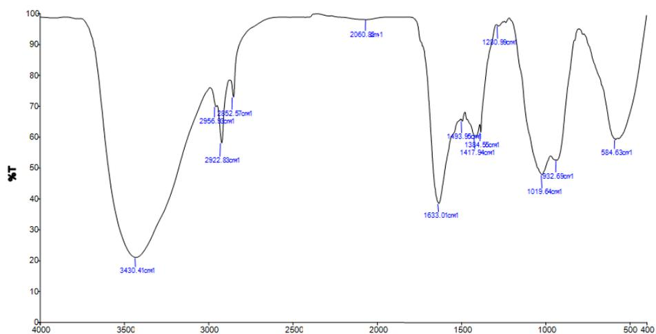
Fig. 3. FT-IR Analysis of *Tecoma stans* mediated copper oxide nanoparticles
