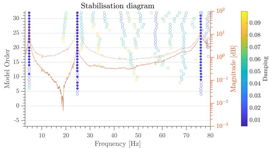
**Figure 9.** Twin spar: stabilisation diagram of the low-input scenario computed with the following parameters:  $\Delta f = 1\%$ ,  $\Delta \zeta = 5\%$  and  $MAC = 0.95$ . The FRF of channels # 3L and 4L are superimposed for further mode visualisation.
