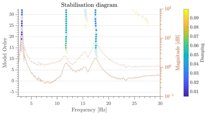
**Figure 21.** Full wing: stabilisation diagrams the low-input scenario computed with the following parameters:  $\Delta f = 1\%$ ,  $\Delta \zeta = 5\%$  and  $MAC = 0.95$ . The FRF of channels #3L and #4L are superimposed for further mode visualisation.
