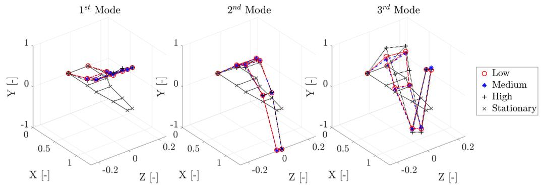
Figure 14. Main spar: mode shapes of the first three vertically dominant modes.
