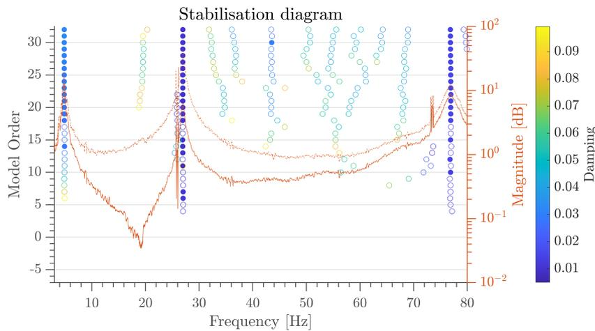
**Figure 13.** Main spar: Stabilisation diagrams showing the low-input scenario computed with the following parameters:  $\Delta f = 1\%$ ,  $\Delta \zeta = 5\%$  and  $MAC = 0.95$ . The FRF of channels # 3L and 4L are superimposed for further mode visualisation.
