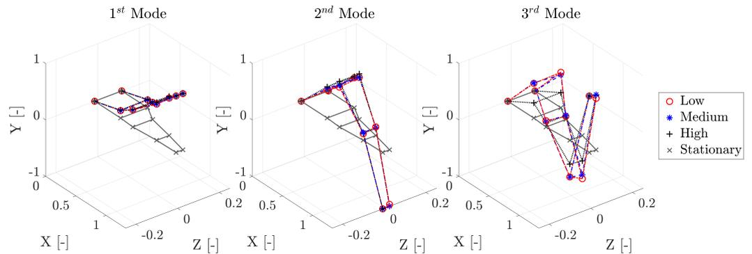
**Figure 10.** Twin spar: mode shapes of the first three vertically dominant modes.
