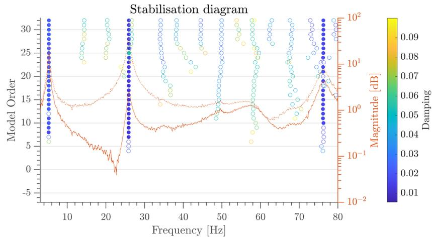
**Figure 17.** Spar and tube: Stabilisation diagrams the low-input scenario computed with the following parameters:  $\Delta f = 1\%$ ,  $\Delta \zeta = 5\%$  and  $MAC = 0.95$ . The FRF of channels # 3L and 4L are superimposed for further mode visualisation.
