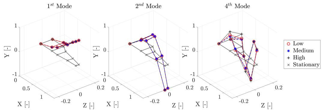
**Figure 18.** Spar and tube: Mode shapes of the first three vertically dominant modes.
