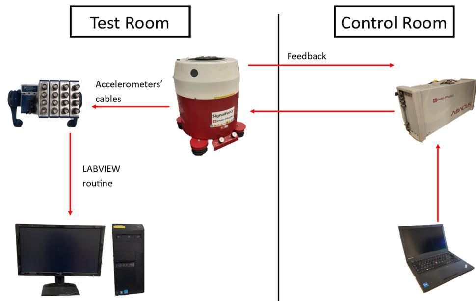
**Figure 7.** Testing setup.
