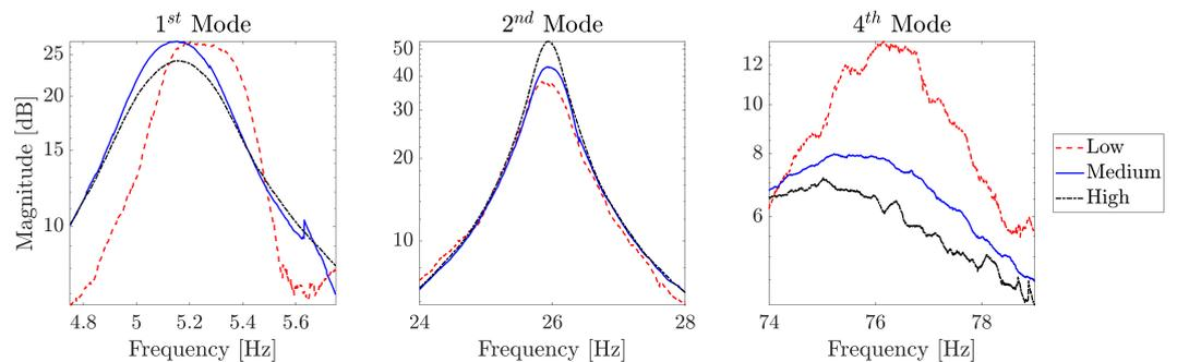
**Figure 19.** Spar and tube: Comparison of the FRFs of channel #4L for the two input scenarios near resonances.
