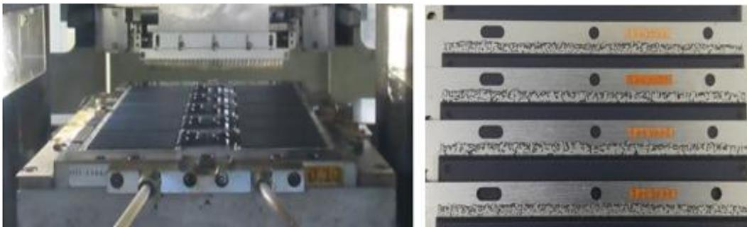
Fig. 11. Strip condition for package sticking validation
